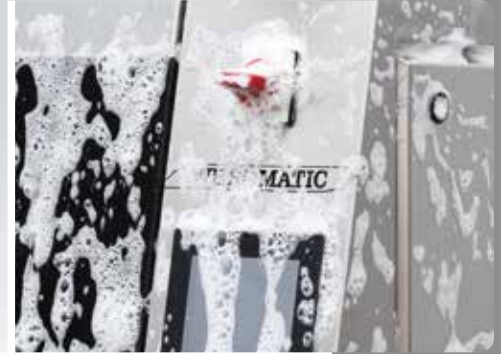
WEBOMATIC CleanDesign®: stainless steel and non corroding materials guarantee all around wash down ability
